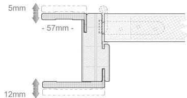
44mm thick Leaf with straight edge, perimeter frame in fir finger joint, internal panel in carboard treated in honeycomb and covers in 4mm mdf. Rimmed on the 3 sides with ABS edge high sealing, also "STOP-WATER" system treatment to ensure water humidity resistance.
