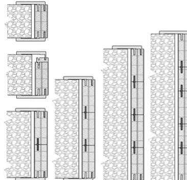
Cased opening Body frame with 90x10mm telescopic casing (jamb)
