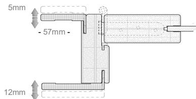
44mm thick five-layer blockboard with 3mm rounded corners; coated using only polyurethane glue which guarantees maximum gluing and waterproofing safety. Laminated glass 4+4mm.
