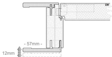
Leaf th. 44mm. with 10 x 10 coplanar edge, finger joint spruce perimeter frame, treated honeycomb cardboard interior and 4mm mdf covers
