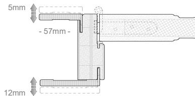
44mm thick Leaf with straight edge, perimeter frame in fir finger joint, internal panel in carboard treated in honeycomb and covers in 8mm mdf. Engraved and varnish with a high resistance to scratches and color change.
