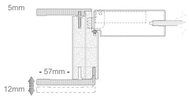
Solid wood blockboard with five layers or honeycomb, 44 mm thick, with 10x10mm coplanar edge; coated using only polyurethane glue which guarantees maximum gluing and waterproofing safety. Laminated glass 4+4mm.
