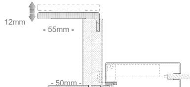
Solid wood blockboard with five layers or honeycomb 44mm thick, 10x10mm coplanar edge; coated using only polyurethane glue which guarantees maximum gluing and waterproofing safety. Laminated glass 4+4mm. Waterproof mechanical PVC seal.
