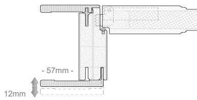
Leaf th. 44mm with 10 x 10 coplanar edge, finger joint fir perimeter frame, treated honeycomb cardboard interior and 8mm MDF covers, engraved and painted with acrylic paints with high resistance to scratches and color change.
