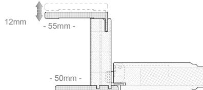
Leaf th. 44mm. With 10x10mm coplanar edge, finger joint fir perimeter frame, treated honeycomb cardboard interior and 8mm mdf covers, engraved and painted with acrylic paints with high resistance to scratches and color change. Waterproof mechanical PVC seal.
