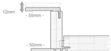
44mm thick Leaf with straight edge, perimeter frame in fir finger joint, internal panel in cardboard treated in honeycomb and covers in 4mm mdf. Rimmed on the 3 sides with ABS edge high sealing, also "STOP-WATER" system treatment to ensure water humidity resistance.
